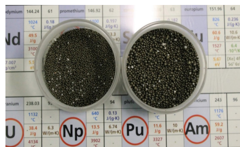
Appearance of high-strength glass-ceramic proppants
